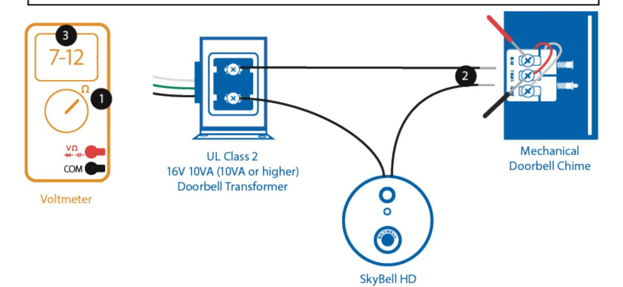
STEP 5 Unscrew Transformer screws to disconnect both wires from Transformer.
